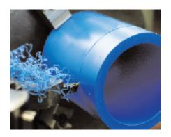
This is not possible with many competitive bearings that are moulded to 'standard' sizes and do not provide overbuild for machining on site as required. Plant and
